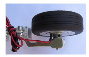
Step 2: Connect two brake wheels' wire into PC-board, and the signal wire into the receiver:
